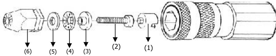
**(1.) Assemble the bearing set & mandrel (parts 2,3,4,5) shown in the figure above.**
